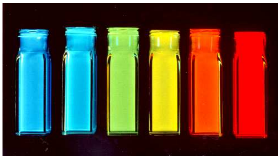
Figure 1.2: Photograph of the size dependent emission spectra of both HgS (top) and CdSe (bottom) quantum dots. Small quantum dots absorb and emit blue/green light, larger dots absorb and emit red light.
