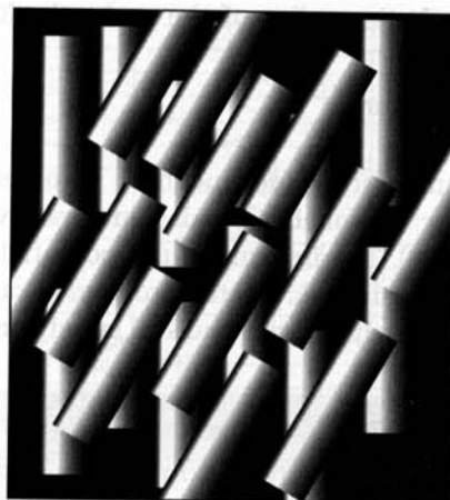
Fig 16.27 The arrangement of molecules in the cholesteric phase of a liquid crystal. Two layers are shown; the relative orientation of these layers is repeated in successive layers, to give a helical array of molecules.
