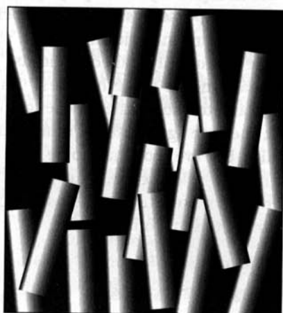
Fig 16.26 The arrangement of molecules in the nematic phase of a liquid crystal.
