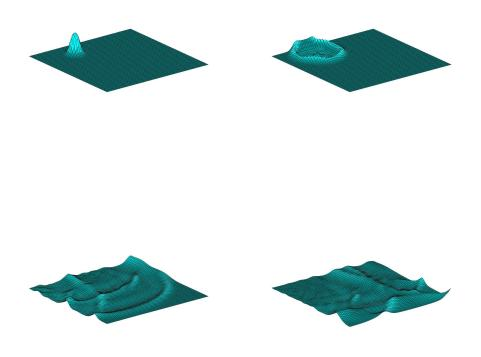
Figure 16.3. A water drop initiates a wave that reflects off the boundary.
