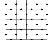
**Figure 16.2.** The first stage computes values that represent the solution at the midpoints of the edges in the finite difference grid.
