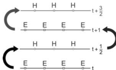
Figure 5.2 Arrangement of the electric- and magnetic-field components with the leapfrog scheme for a 1D case.
