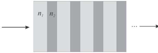
Figure 10.4 Schematic diagram of a 1D periodic layered structure (1D-PBG). Propagation is along the horizontal direction.
