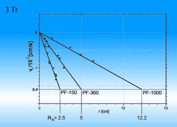
The radial velocity of the plasma sheath is the linear function of radius (r)
